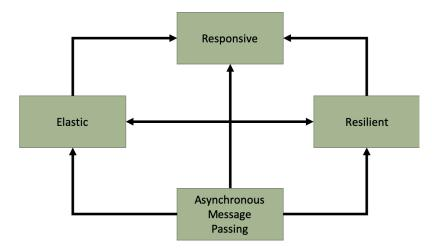
Microservices as part of reactive systems interact using *messages*. The location and temporal decoupling, promoted by this interaction mechanism, enable numerous benefits such as:
